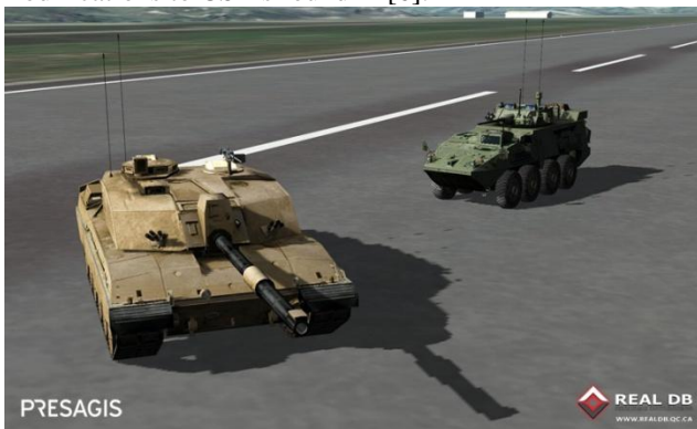
Figure 3: An improvement compared to Figure 1. In this image the cascaded shadow map solution captures shadowing information using four shadow maps versus just one. The result yields a substantial increase in detail in the tank shadow.
