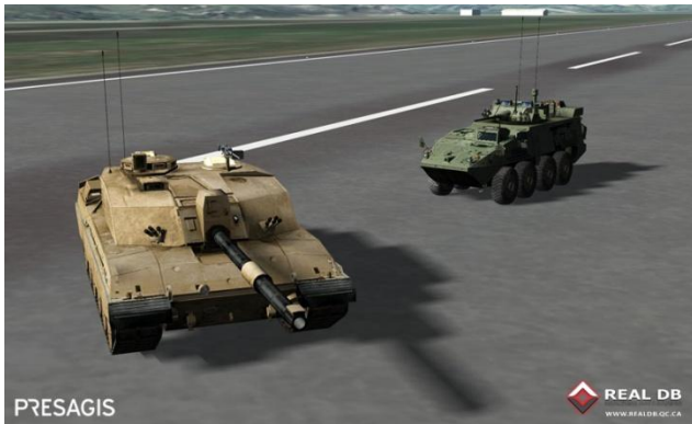
Figure 1: An example of perspective aliasing. While the shadow map resolution of 512x512 might be sufficient for the vehicle in the background, the shadow cast by the tank in the foreground lacks detail. Cascaded Shadow Maps, discussed later, can be used to improve this issue.
