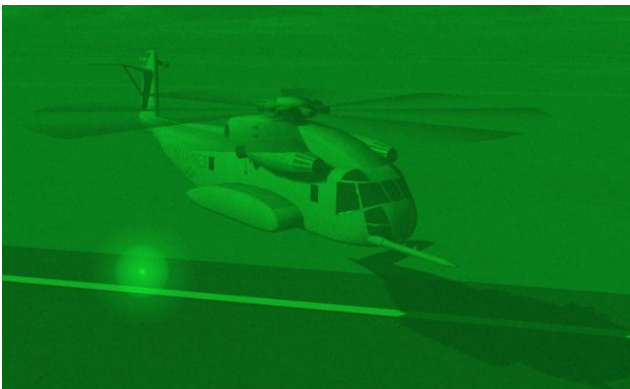
Figure 5: Shadows in NVG look like those in the visible spectrum. Notice both the self-shadowing of the
