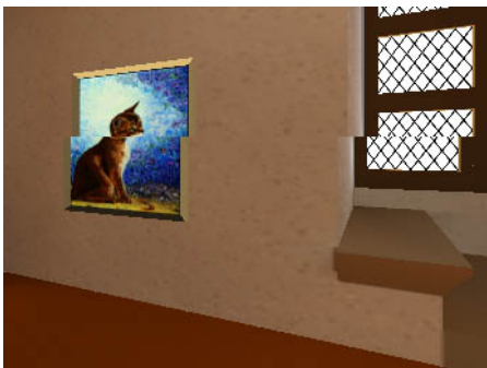
Figure 8: Horizontal image tearing (the image is being updated at the same time it is being drawn)
