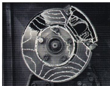
Brake disc vibration at 2.1 kHz and 18 rpm using electronic speckle pattern interferometry
