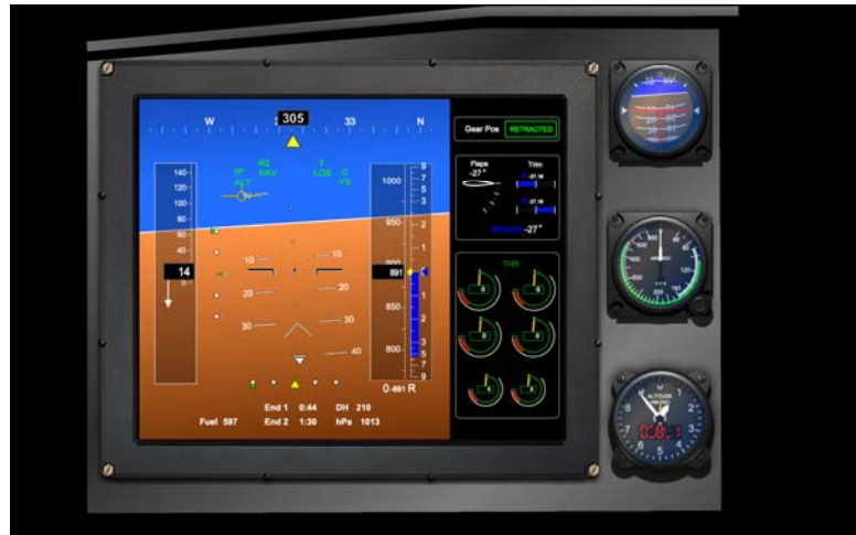
Figure 1. Primary Flight Display created with VAPS XT
