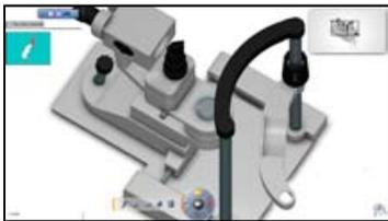
Positioning relationships are proposed on-the-fly using visual highlights as you approach parts or sub-assemblies. CATIA Live Compose makes it possible to build innovative proposals quickly in a 3D brainstorming spirit.
