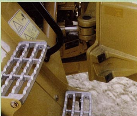
Wide steps with good grip and a rounded handle – as seen on Caterpillar's 730 articulated truck
