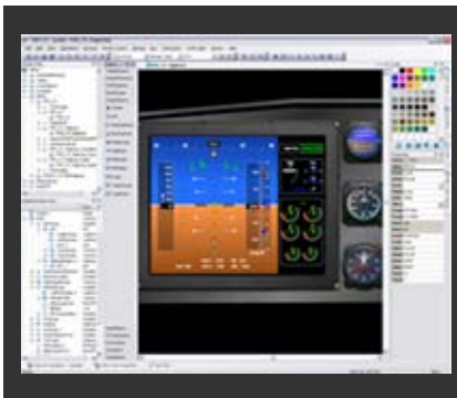
Cockpit display designed using the Human Machine Interface Tool
