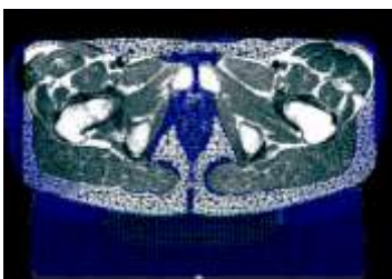
Figure 1: Abaqus FEA overlay of MRI image was used to validate the body/foam interaction model. Shown is an FEA-mesh of a cross-section of a human pelvis MRI (upper grey and white area) resting on a foam cushion (square purple meshed portion at bottom). Using imaging techniques in this way is key for verifying the accuracy of biomechanical modeling of living subjects.
