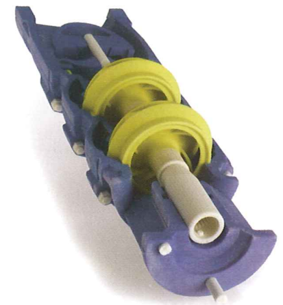
▲ Figure 2b: An example of the level of detail you can achieve on the EOS P100 Formiga. These damping springs built very successfully and are under a millimetre thick.
