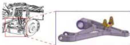
Figure 2: Suspension system assembly and control arm.
