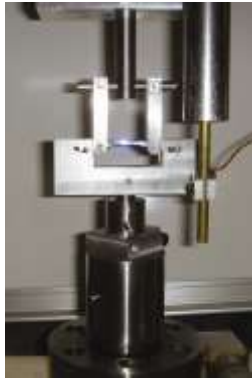
Nitinol four-point bend test sample with moiré interferometry diffraction grating used for material characterization.
