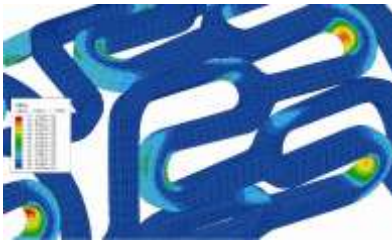
Strain contour data from a stent fatigue analysis. convincing them that they represent actual experience.
